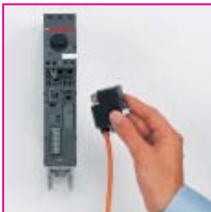
Connection to the bus by plug connection
